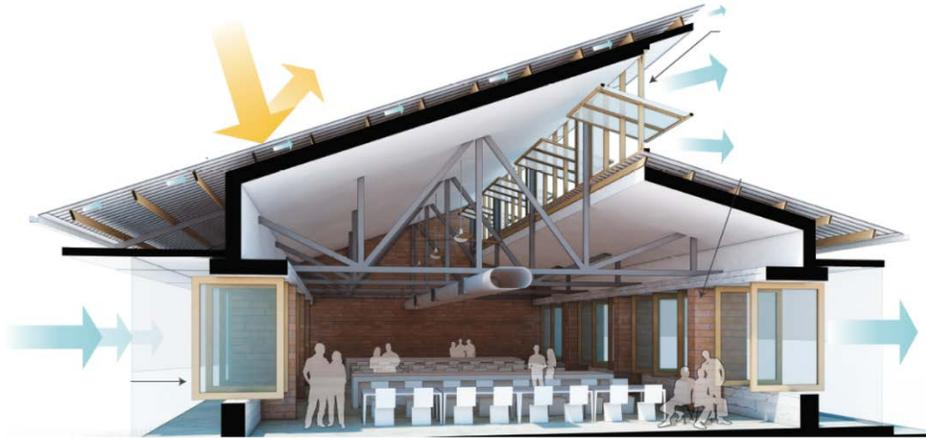
**Figure 1: Artist's initial rendering of the conceptual design of the DLC building by Gensler.** Yellow arrows show reflection of solar radiation; blue arrows show wind flow and cross ventilation.
