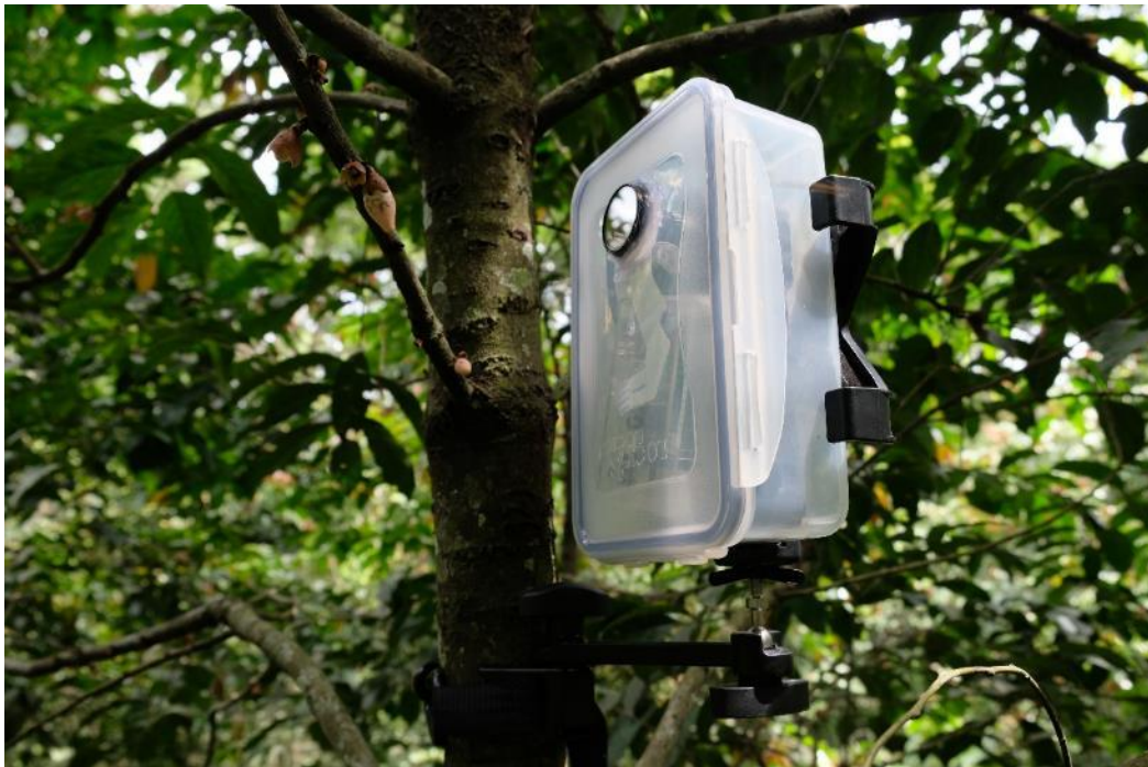
Figure A.9. The camera developed during the project to record movies of insect pollinating the flowers. The camera is mounted on the tree, focusing on a flower from before its anthesis until its dead. Image by V. Deblauwe.
